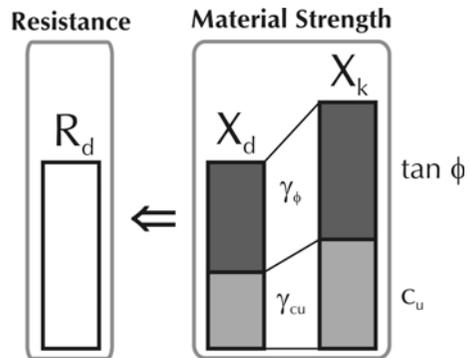
**Figure 85.** Hierarchy of material strengths and resistance when factors are applied to material properties only
