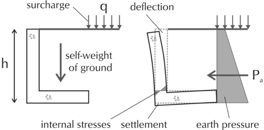
Figure 80. Actions (left) and effects (right) for L-shaped gravity retaining wall
