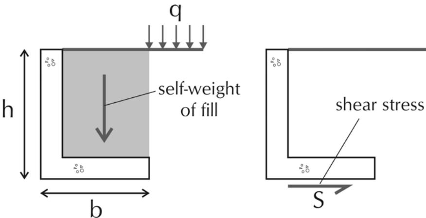
**Figure 81.** Sliding resistance of L-shaped gravity retaining wall
