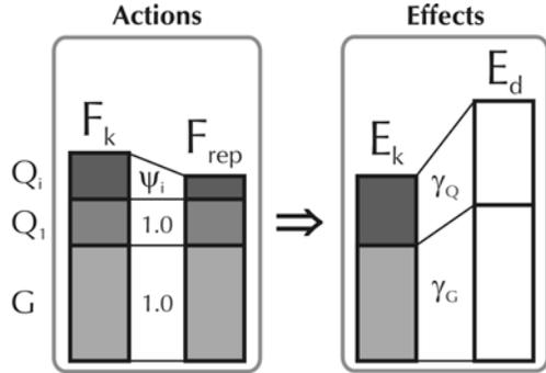
**Figure 84.** Hierarchy of actions and effects when partial factors are applied to action effects
