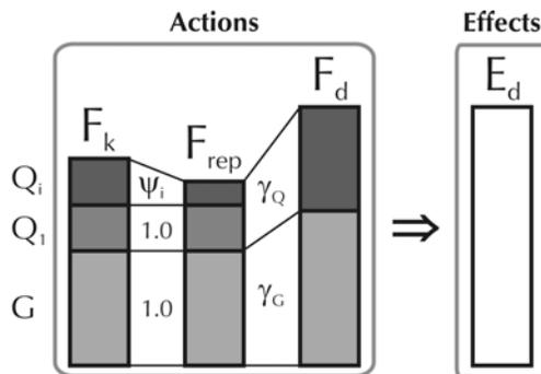
**Figure 83.** Hierarchy of actions and effects when partial factors are applied to actions
