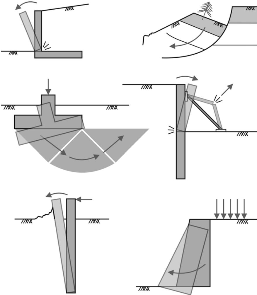
Figure 79. Examples of ultimate limit states of strength
