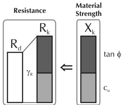
**Figure 86.** Hierarchy of material strengths and resistance when factors are applied to resistance only
