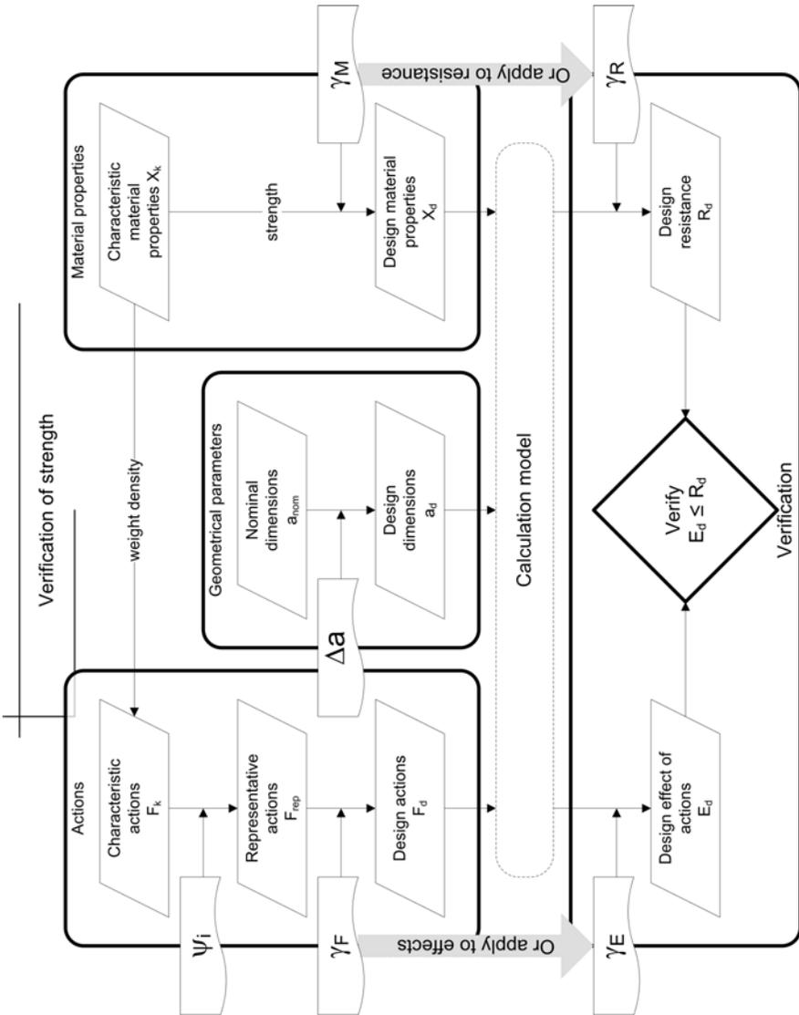
Figure 82. Overview of verification of strength
